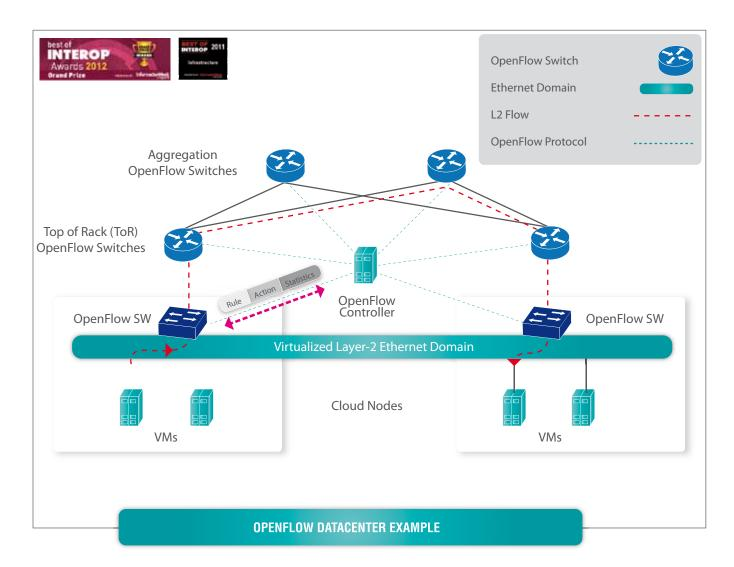
ProgrammableFlow resolves most of traditional networks issues or constraints while simplifying Network management and maintenance (Software control) and brings the required flexibility for the setup of ITaaS.
