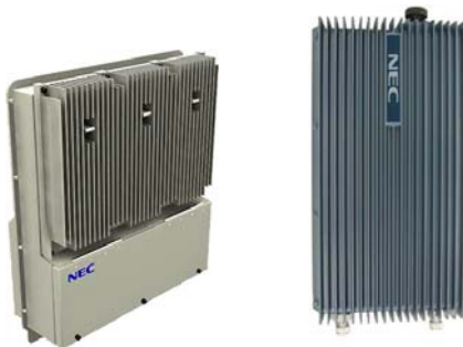
Figure 3: Compact and Fanless LTE Base Stations
