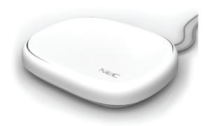
FP1624 small cell is an indoor base station for small to medium enterprises. It supports HSPA+ data rates while supporting up to 16 simultaneous calls.
