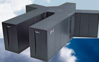
SX-4 Multi node (> 10 nodes) processor with CMOS and air-cooling
